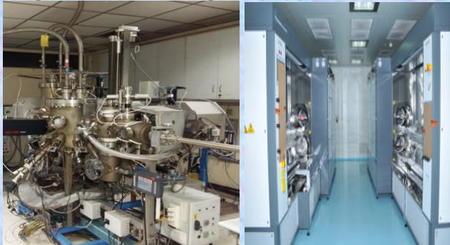
UHV RF-plasma assisted Diffusion oxidation & Molecular Beam Epitaxy PECVD system
